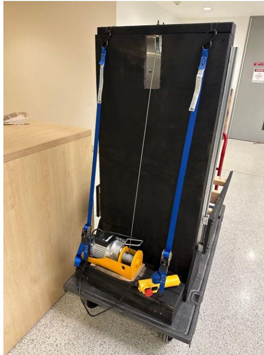
Figure 6.22 - Electric winch attached to the elevator frame
